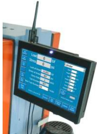
If selected at the operator's console, the system queries the operator as to the "break type" observed before proceeding to set up for the next test. The observed "break type" is recorded against the test id number.
